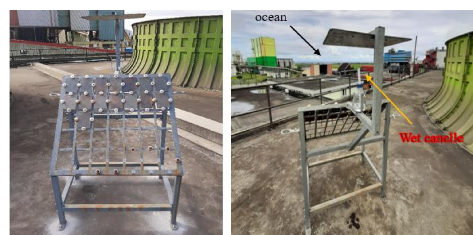
Figure 2. Exposure of bare CS specimens for a period of 14 months.
