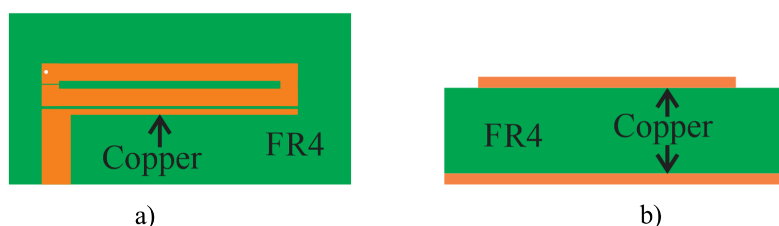
Figure 1. (a) Top view and (b) front view of a rectangular resonator.
