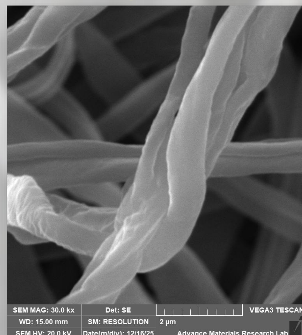
Result 1: SEM demonstrated uniform nanofiber morphology
