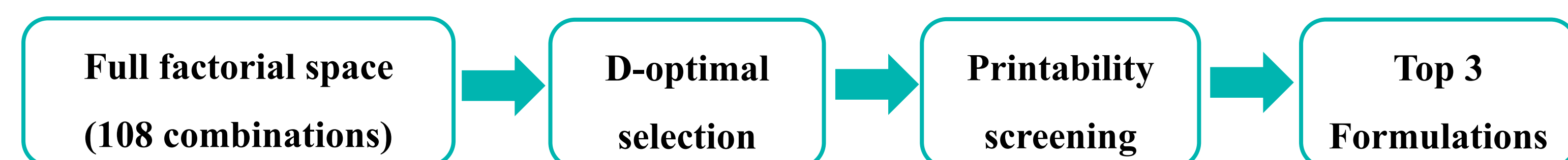
Figure 2 Workflow of D-optimal experimental design for printing ink formulation screening.
