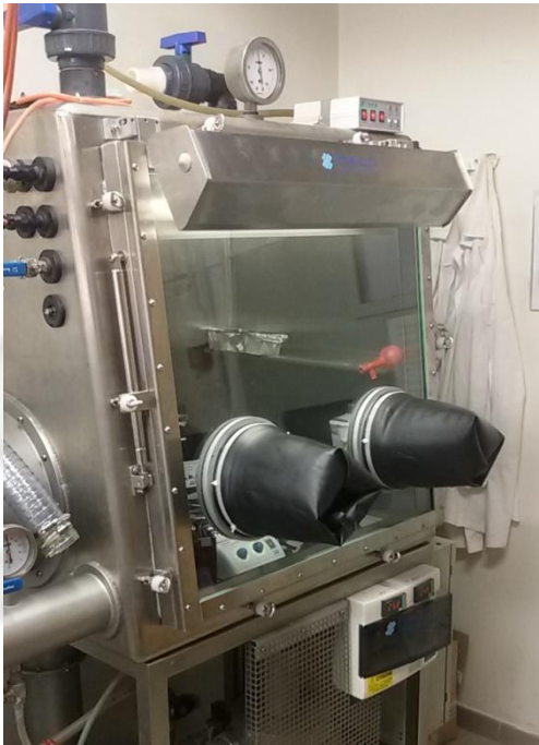
Glove Box to prevent moisture contamination of the IL
