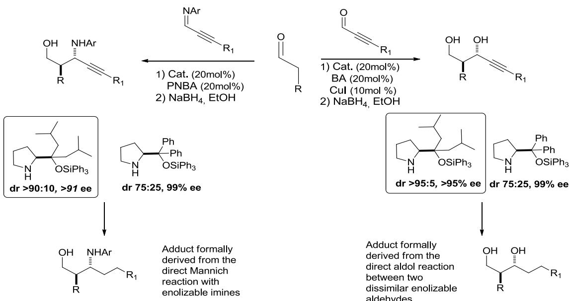
This study uncovers a new case of chiral enamine catalysis in which  $\alpha,\alpha$ -dialkylprolinol silyl ethers perform better than their parent  $\alpha,\alpha$ -diaryl analogs. The resulting densely functionalized adducts may be transformed into more complex systems taking advantage of the chemistry of the triple bond.
