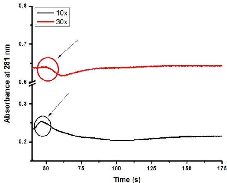
Time traces obtained for the reaction of 0.02 mM GSH and 10 and 30-fold excess of the concentration of  $[\text{ZnCl}_2(\text{terpy})]$  complexes at pH 7.38 (the arrows point to the rise and fall in absorbance).
