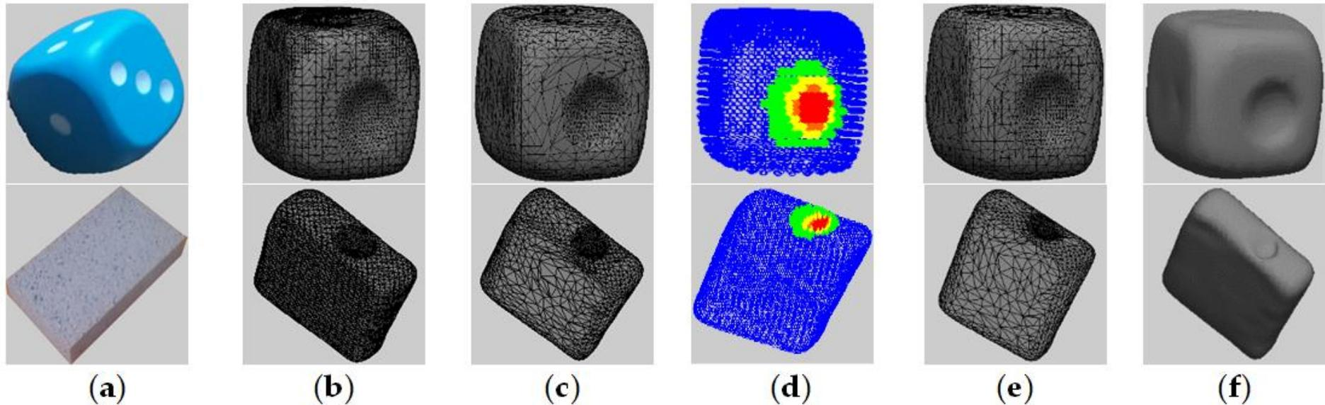
(a) initial object; (b) initial object mesh; (c) mesh with higher density in the deformed area; (d) stratified sampled data for neural-gas mapping; (e) neural-gas-tuned simplified object mesh and (f) final object model.
