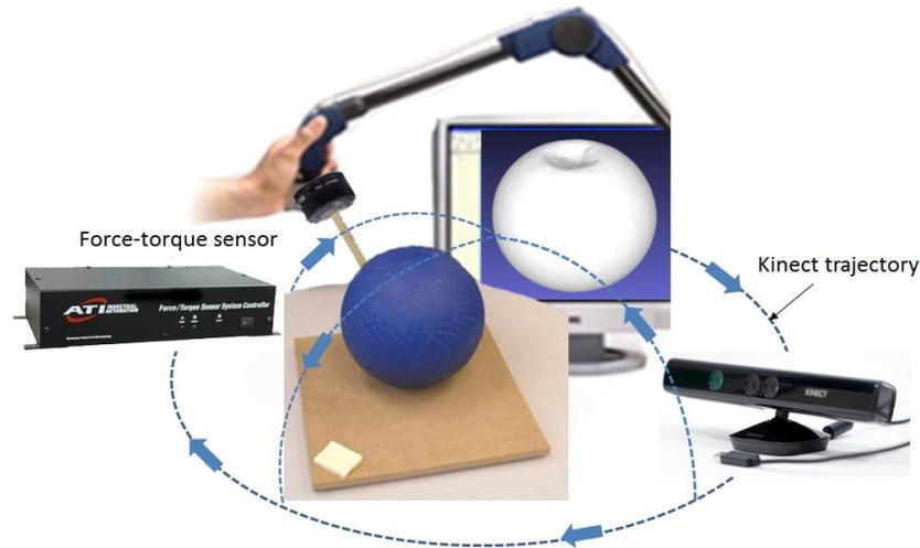
Acquisition platform for soft object deformation behavior including a Kinect sensor to collect 3D geometry data and an ATI force-torque sensor to measure the force magnitude;
