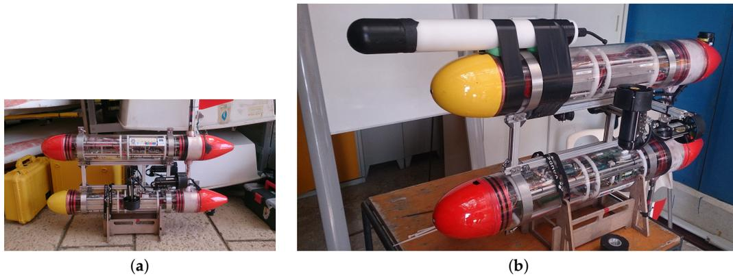
**Figure 3.** (a) Photo of the red MEDUSA as operated in this trial and (b) turned upside down position with DAVS attached to it.
