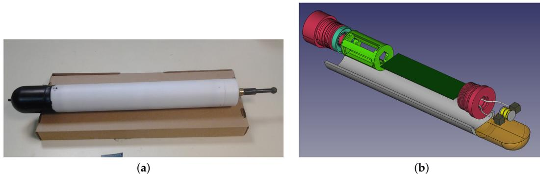
**Figure 1.** (a) Photo of DAVS and (b) exploded view of DAVS in 3D solid modelling, showing the Delrin container (white half tube), the acoustically active part (dark yellow), the two accelerometers (gray blocks), the hydrophone (yellow cylinder), the threaded caps (pink), the electronics (dark green block) and the battery pack (light green).
