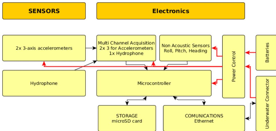
**Figure 2.** DAVS electronic overview: The hydrophone and the two accelerometer signals are acquired on the multi-channel acquisition board, 7 channels in total. The micro-controller receives data from multi-channel acquisition board and stores it in the SD card. Non acoustic sensors give the roll, pitch and heading of the device. Power can be obtained from internal batteries or from external source through a power cable.
