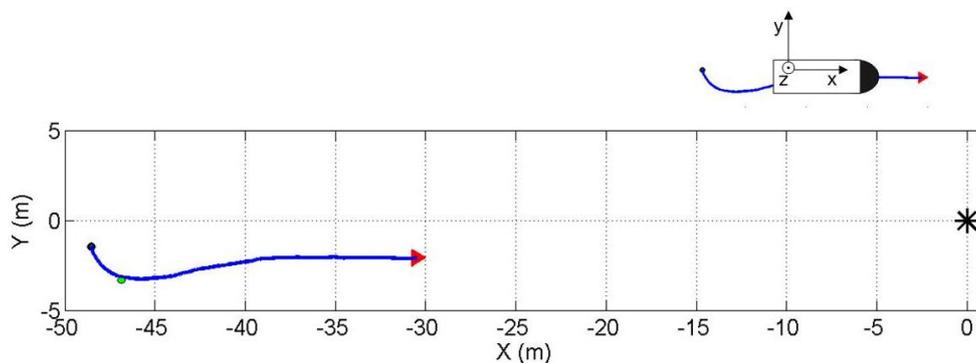
**Figure 4.** Sailed track of the AUV towards the source (black asterisk). The black dot indicates the starting point and the arrow the end point for the estimation. The illustration on the top right corner of the figure shows the sensor coordinate system with respect to the track.
