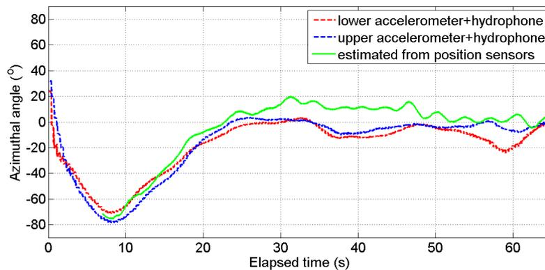
**Figure 5.** Estimation of sound azimuth direction of the sound relative to AUV sailing from the track shown in Figure 4, as computed from the lower (red curve) and the upper (blue curve) accelerometer. The green line gives the source azimuth estimate as derived from the AUV positional sensors starting from the point of the track indicated with the green dot in Figure 4.
