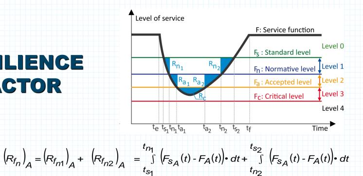
$$\left( R_{f_a} \right)_A = \left( R_{f_{a1}} \right)_A + \left( R_{f_{a2}} \right)_A = \int_{t_{n_1}}^{t_{a_1}} \left( F_{n_A}(t) - F_A(t) \right) \cdot dt + \int_{t_{a_2}}^{t_{n_2}} \left( F_{n_A}(t) - F_A(t) \right) \cdot dt$$
