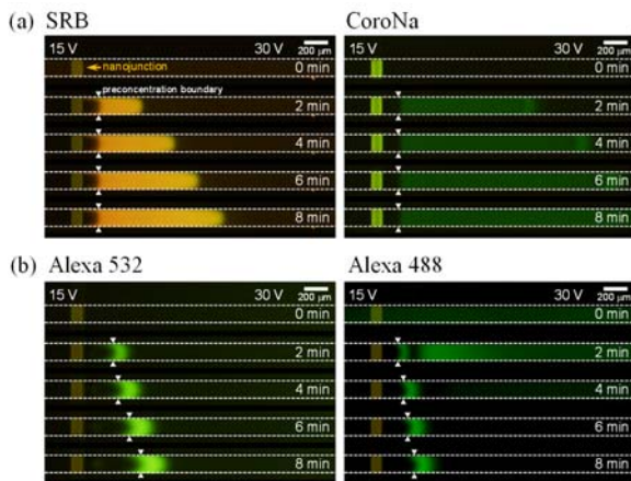
Fig. 3 Time-lapse images of each preconcentration behavior of (a) SRB and CoroNa (stacking regime) and (b) Alexa 532 and Alexa 488 (propagating regime). Two opposite white triangles designated the preconcentration boundary of each analyte.
