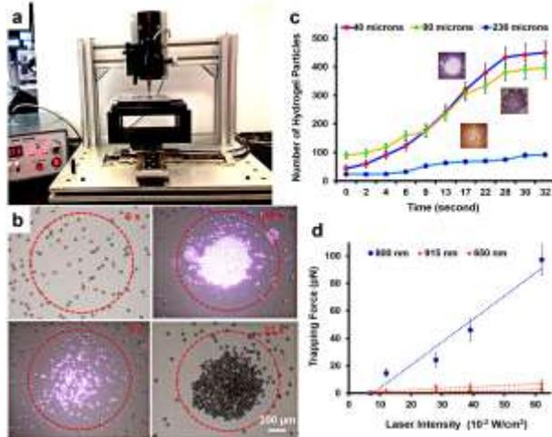
Figure 4. High-throughput light assembly of microparticles by controlling the laser equipped in an automatic stage
