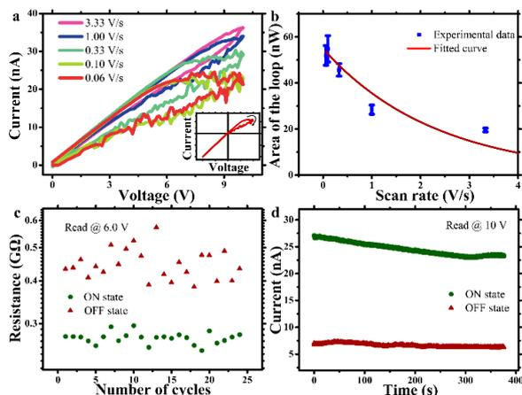
Fig. 2 A conical nanochannel (6 nm in tip diameter) immersed in the mixture electrolyte with [BMIM][BF<sub>4</sub>] molar fractions of 0.07. (a) I-V characteristics with different scanning rate. (b) The area of hysteresis loops as a function of scan rates. (c) Retention time of the ON/OFF state current of nanofluidic memristor at a positive voltage of 10 V. (d) ON/OFF resistances plotted as a function of the number of cycles.
