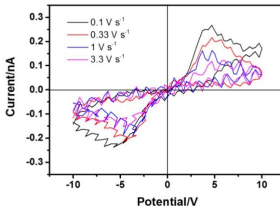
Fig. 4 A conical nanochannel (12 nm in tip diameter) immersed in the mixture electrolyte with TBLs molar fractions of 0.3. under different scan rates.
