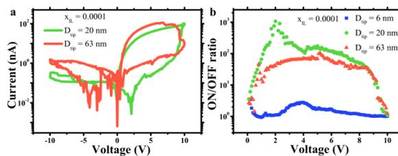
Fig. 3 (a) The resistance at ON/OFF state as a function of bias voltage, with 20 nm and 63 nm tip opening size at  $x_{IL} = 0.0001$ . (b) The ON/OFF resistance ratio as function of positive bias voltage that has better ratio than the negative voltage.
