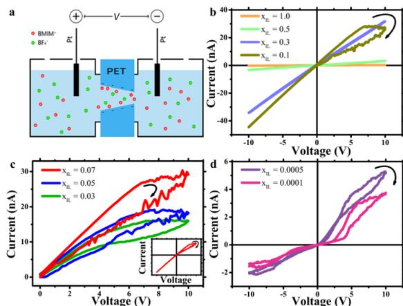
Fig.1 (a) Schematic illustration of the experimental setup with ionic transport through a conical nanochannel. The electrolyte was mixed solution of [BMIM][BF<sub>4</sub>] and water.  $x_{IL}$  indicates mole fraction of [BMIM][BF<sub>4</sub>]. (b), (c) and (d) were typical I-V curves using a conical nanochannel of 6 nm tip openings immersed in the [BMIM][BF<sub>4</sub>]-water mixed electrolyte solution. Arrow denotes switching direction.
