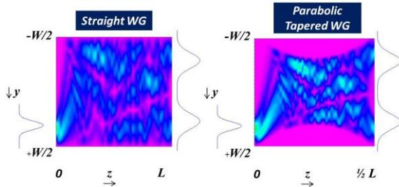
Fig. 1. Schematic illustrating the difference between straight and parabolic tapered waveguide.
