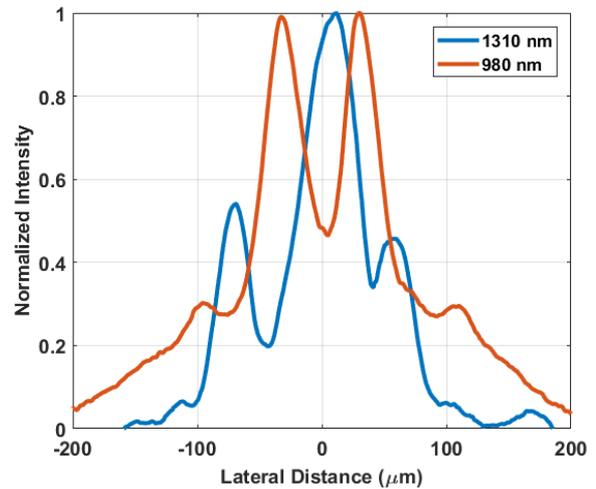
Fig. 5. Measured output intensity profile of the MMI splitter at input wavelengths of 1310 nm and 980 nm.
