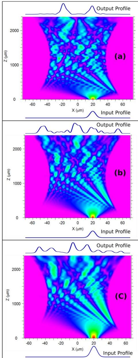
Fig. 2. Simulation contour plots for the field inside the MMI waveguide and the corresponding input and output field intensity profiles for (a) 2200 nm wavelength at which it acts as a 1x2 splitter, (b) 1300 nm wavelength at which it acts as a 1x3 splitter and (c) 980 nm wavelength at which it acts as a 1x4 splitter.
