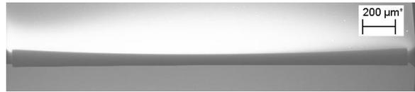
Fig. 3. Scanning electron microscope (SEM) image of the fabricated splitter on Si.
