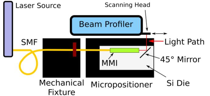
Fig. 4. Schematic diagram of the setup used in structure characterization.
