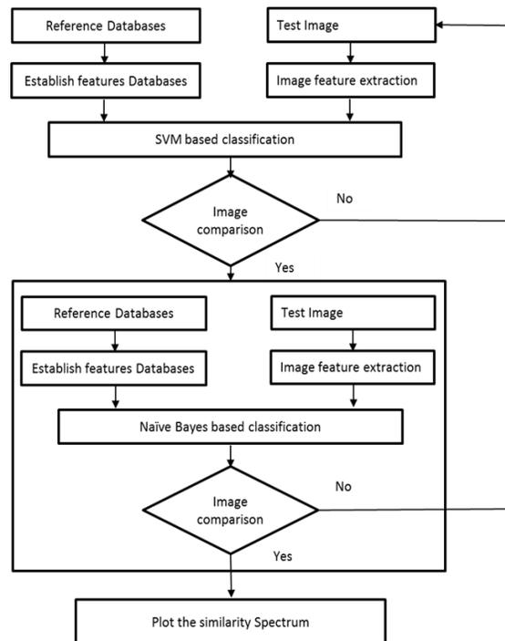
Fig. 3. Flowchart of classification algorithm.
