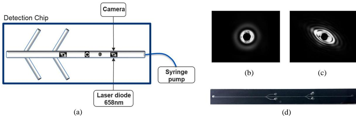
Fig. 1. (a) Detection Micro-fluidic Chip. (b) Image of Cryptosporidium. (c) Image of Giardia. (d) Photo of the Chip.
