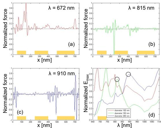
Fig.1 Gradient force produced by a plasmonic nanopost: (a)  $\phi = 100$  nm, (b) 150 nm, and (c) 200 nm. The force was calculated at the resonant wavelength shown. (d) shows the normalized maximum electric field strength in a spectral band of  $\lambda = 650 \sim 1100$  nm.
