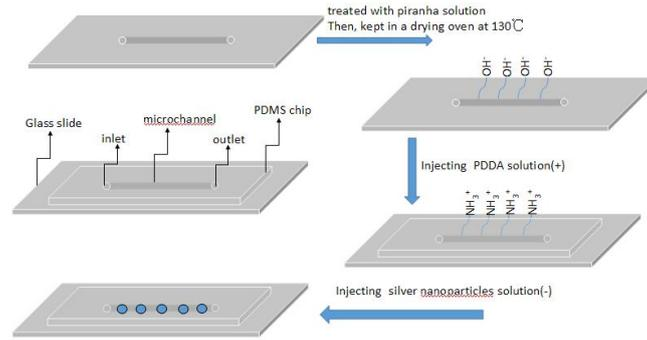
Fig. 1. Schematic diagram of the preparation of SERS substrate in microfluidic channels.
