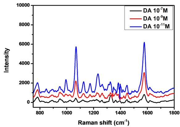
Fig. 3. SERS spectrum for different DA concentration.
