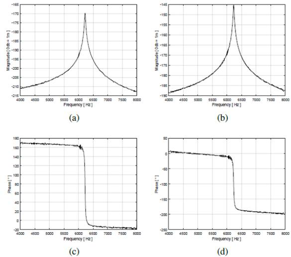
Fig. 4 (a) Frequency response of top actuator (b) Frequency response of bottom actuator (c) Phase response of top actuator (d) Phase response of bottom actuator
