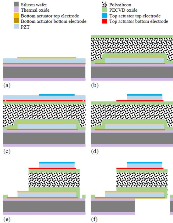
Fig.1 Fabrication process steps of the bimorph PZT micro-cantilever actuator
