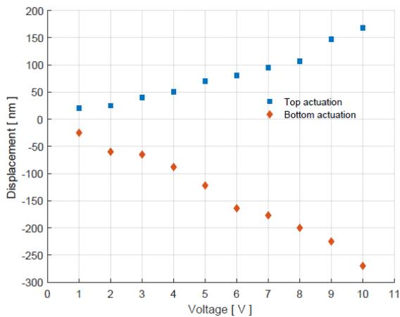
Fig. 3 Static deflection measured by Polytec MAS-500
