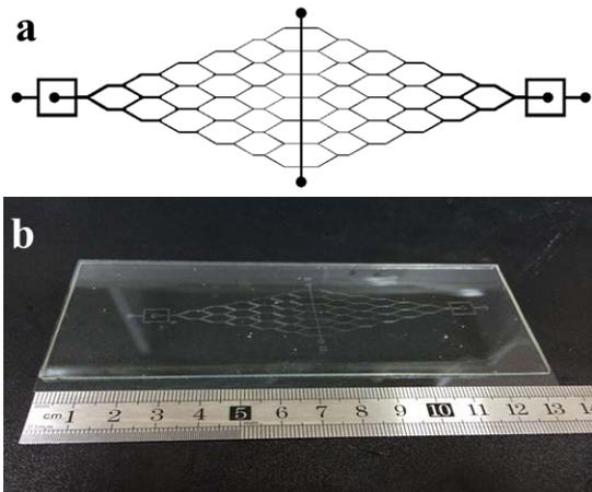
Fig.1 (a) the CAD drawing of the Y shaped microchannel and (b) photo of the fabricated chip.
