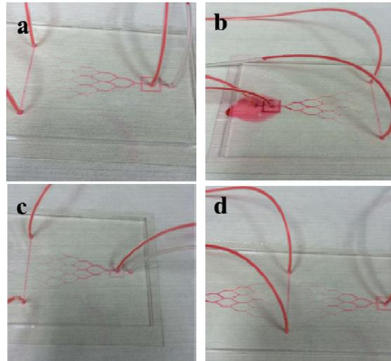
Fig.4 Leak test of PDMS chip bonding only by polaroid bonding (a, b) and polaroid bonding combined thermal bonding (c, d) at different flow rates: (a, c)  $200 \mu\text{L}\cdot\text{h}^{-1}$ , (b)  $250 \mu\text{L}\cdot\text{h}^{-1}$ , (d)  $1000 \mu\text{L}\cdot\text{h}^{-1}$ .
