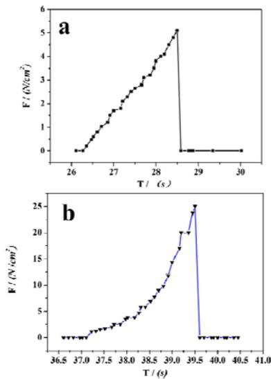
Fig.3 The adhesion force between PDMS and glass when PDMS-glass bonded (a) only by polaroid bonding, (d) by polaroid bonding and thermal bonding.
