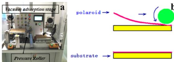
Fig.2 (a) the polaroid bonding machine used in this study and (b) the schematic illustration of the machine's working principle.
