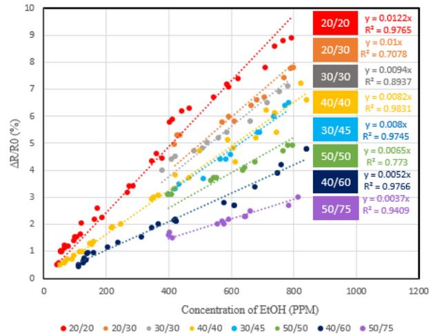
Fig. 6 The sensitivity of different layout sensors with response to ethanol concentration. The numbers indicate line width/electrode gap ( $\mu\text{m}$ ).
