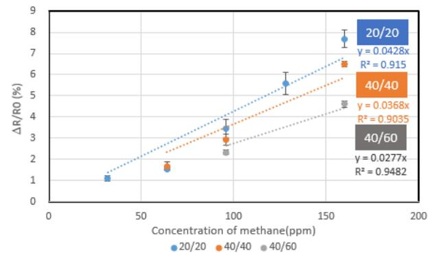
Fig. 7 The sensitivity of different layout sensors with response to methane concentration. The numbers indicate line width/electrode gap ( $\mu\text{m}$ ).
