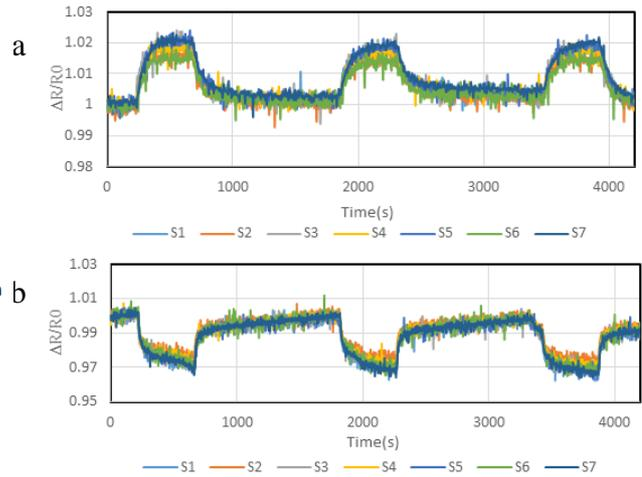
Fig. 5 When the sensor is coating with PNVP, (a) resistance increases upon exposing in ethanol and (b) decreases in methane on the contrary.
