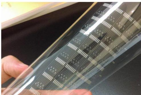
Fig. 3 The gas sensor array printed on PET.
