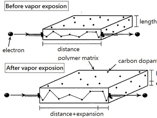
Fig. 1 The mechanism of resistive gas sensor using polymer and carbon black mixture as sensing material.
