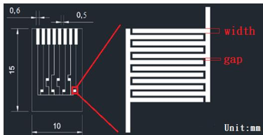
Fig. 2 Sensor chip layout and the magnified interdigitated electrode with line width and electrode gap illustrated.
