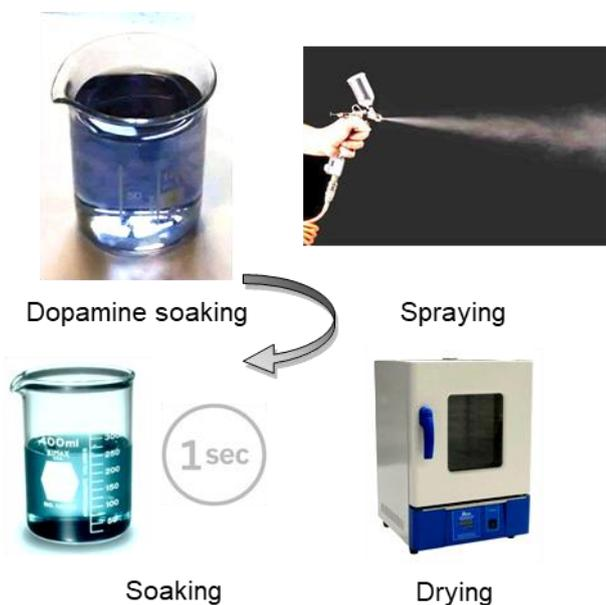
Fig. 3 Process flow for preparing the  $\text{TiO}_2$  thin film on the black PMMA substrate at room temperature. It starts with soaking the PMMA sheet in dopamine and then spraying P25  $\text{TiO}_2$  solution. After drying in the oven, the PMMA sheet is soaked in chloroform.
