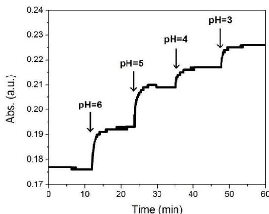
Fig. 3. The real-time pH monitoring of a saliva sample (from a normal person) using a PANI-GNPs-glass biosensor.
