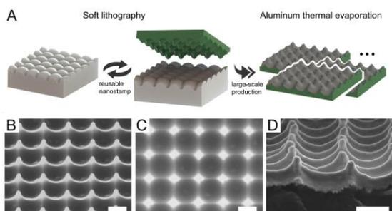
Fig. 2. Schematic illustration of the fabrication procedure of Al NPA nanostructures by ESL and subsequent Al deposition. The elastic nanostamp is molded from a NPA fabricated through EBL and electrochemical etching, and used repeatedly for high throughput of NPA substrates composed of transparent polymer and Al nanostructures.
