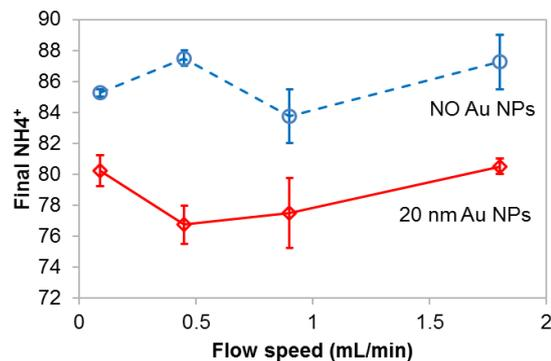
Fig. 4. Reserved  $\text{NH}_4^+$  after treatment for various water pumping flow speed with and without Au NPs fixed in MOFC reactor.
