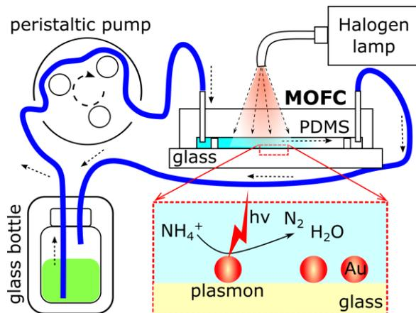
Fig. 1. Schematics of the MOFC reactor.
