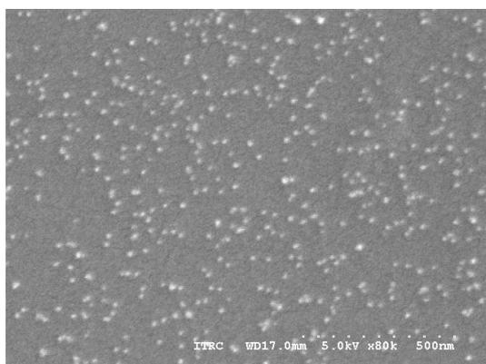
Fig. 3. Au NPs fixed on glass substrate.
