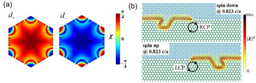
Fig. 1 Transverse spin angular momentum and unidirectional robust transport in silicon topological photonic crystals. (a) Ellipticity angle distribution of pseudo-spin up state  $d_+$  and pseudo-spin down state  $d_-$ . The rod radius is  $0.33b$ , where  $b$  is the distance between the nearest rods. (b) Unidirectional pseudo-spin down and up edge states, which is excited by the right-handed circularly-polarized (RCP) and left-handed circularly-polarized (LCP) sources, respectively.
