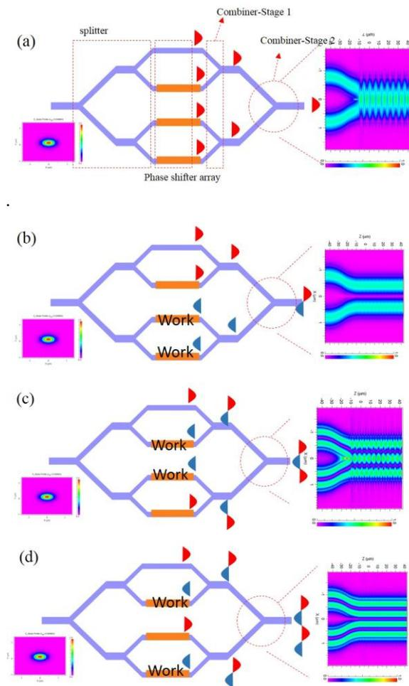
Fig. 2 Simulation result of optical mode converter output mode is (a) TE<sub>0</sub> mode; (b) TE<sub>1</sub> mode; (c) TE<sub>2</sub> mode (d) TE<sub>3</sub> mode
