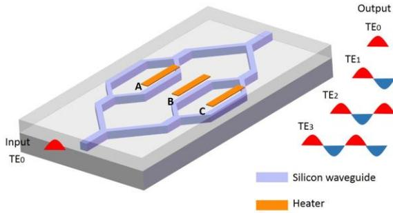
Fig.1 Schematic diagram optical mode converter.
