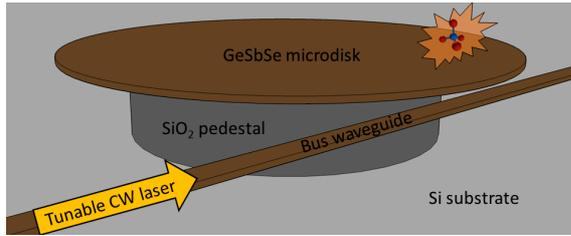
Fig.1 Schematic of a suspended microdisk cavity structure for sensing a target gas molecule in the surrounding air. Brown denotes a  $30\ \mu\text{m}$  radius  $\text{Ge}_{23}\text{Sb}_7\text{Se}_{70}$  microdisk coupled to a bus waveguide, all suspended  $10\ \mu\text{m}$  above a Si substrate by  $\text{SiO}_2$  supports.
