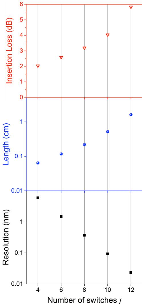
Fig. 3 Projected spectral resolution, interferometer arm length and insertion loss of the dFTIR spectrometer.
