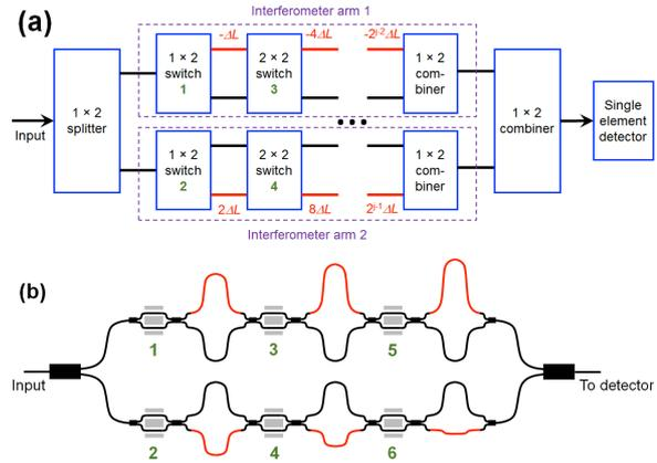
Fig. 2 (a) Block diagram of the dFTIR spectrometer design; (b) schematic layout of a 64-channel dFTIR spectrometer: the waveguide segments of varying lengths different from the standard length are shown in red (not drawn to scale). The green numbers label the  $1 \times 2$  or  $2 \times 2$  switches.
