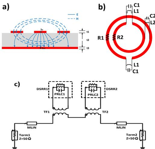
Fig.3 (a) Cross section of a microstrip transmission line with a pair of DSRR and a schematic electromagnetic field distribution, (b) Electrical components of DSRR element, (c) equivalent circuit of the metamaterial sensor.
