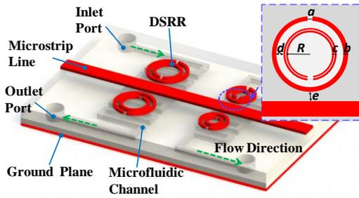
Fig.1 Schematic diagram of the metamaterial micro-fluidic sensor and the size of DSRR.
