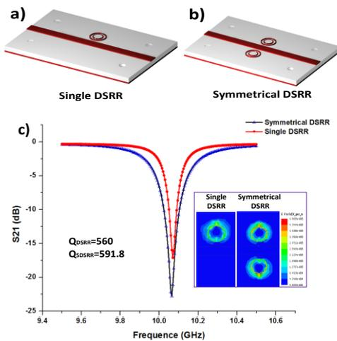
Fig.2 Schematic diagram of metamaterial sensor with (a) single DSRR, or (b) symmetrical DSRR, and (c) simulated results of the DSRR sample and distribution of surface current density (right inset)
