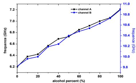
Fig.5 Resonant frequency for ethanol in channel A (black solid) and channel B (blue solid) with different concentrations, from 0% (DI water 100%) to 100%.
