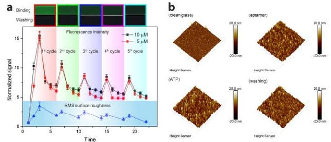
**Fig. 2** (a) Five cycles washing with DI water by using ATP as a target molecule. (b) The AFM images show the change in surface roughness before and after ATP captured by aptamer probes.
