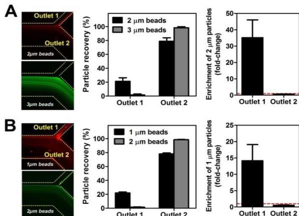
**Figure 3** Average fluorescent composite images and flow cytometry analysis for small particle separation between (A) 2 and 3  $\mu\text{m}$ , and (B) 1 and 2  $\mu\text{m}$  bead mixture using the HiDFF microdevice at optimized conditions. Smaller particles are sorted and highly enriched at the smaller inner wall outlet (outlet 1).
