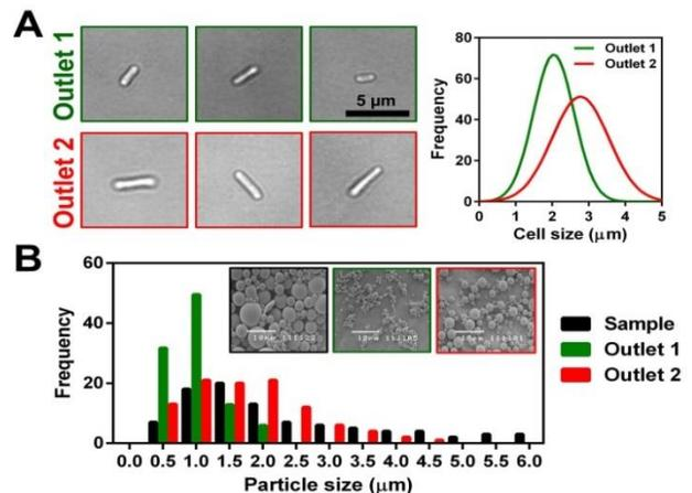
**Figure 4** (A) Size fractionation of bacteria population (*E. coli*) using HiDFF. Smaller *E. coli* are enriched in outlet 1. Size distribution is obtained from ~80-100 measurement in each outlet. (B) Size fractionation of PLGA nanoparticles. Inset SEM images highlight distinct size differences between sample (inlet) and different outlets.
