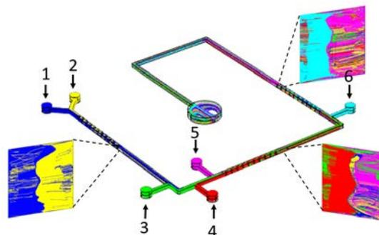
Fig. 6 Simulation results of the microfluidic device with passive mixers using thin barriers for Au nanorods synthesis.
