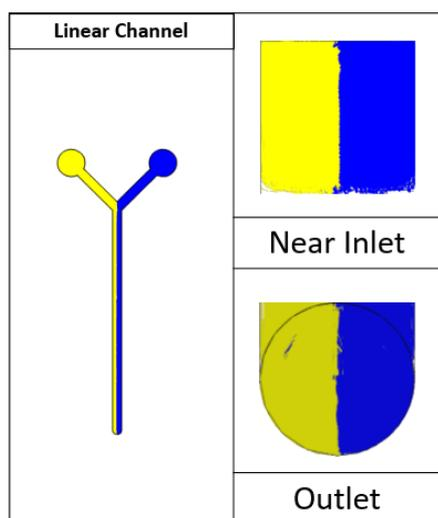
Fig. 3 The magnified top and cross sectional views of a part of microchannel shown in Fig. 2 after mixing of the chemical 1 and 2.
