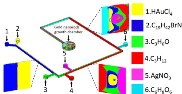
Fig. 2 Mixing simulation results of 6 chemicals for Au nanorods synthesis. Each chemical from 1 to 6 is injected into inlets from 1 to 6 in turn, respectively.
