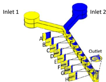
Fig. 4 The mixing simulation results of a part of microchannel with a passive mixer having thin barriers.
