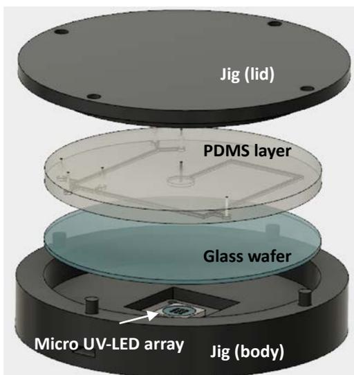
Fig.1 Schematic view of the microfluidic device for synthesis of Au nanorods.
