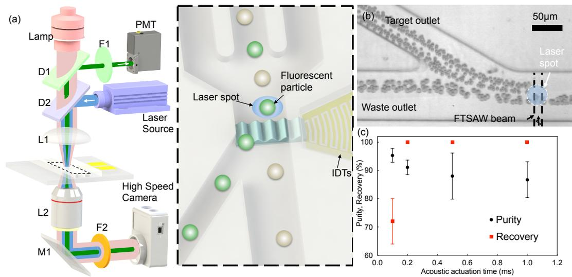
Fig. 1. (a) Schematic illustration of our acoustic fluorescence activated cell sorting (FACS) system. (b) Time-lapsed photos of the particles sorting process based on their fluorescent label. (c) Correlation between the sorting performance (purity and recovery) and the acoustic actuation time of each sorting event.
