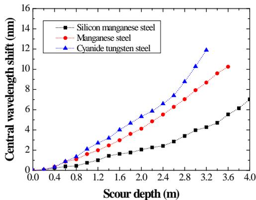
Fig. 2 The central wavelength shift as a function of bridge scour depth for different metal materials.
