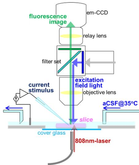
Fig.1 Schematic diagram of the experimental set-up with the laser light irradiation, the electrical microstimulation, and the epi-fluorescence imaging of the cerebral tissue slice perfused with temperature-controlled aCSF.
