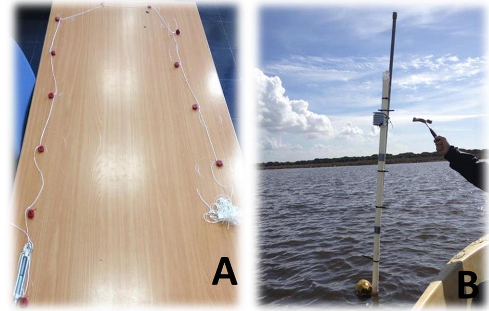
A) Chain of sensors prepared to be installed. B) sensors installed inside a PVC tube in Santa Olalla pond
