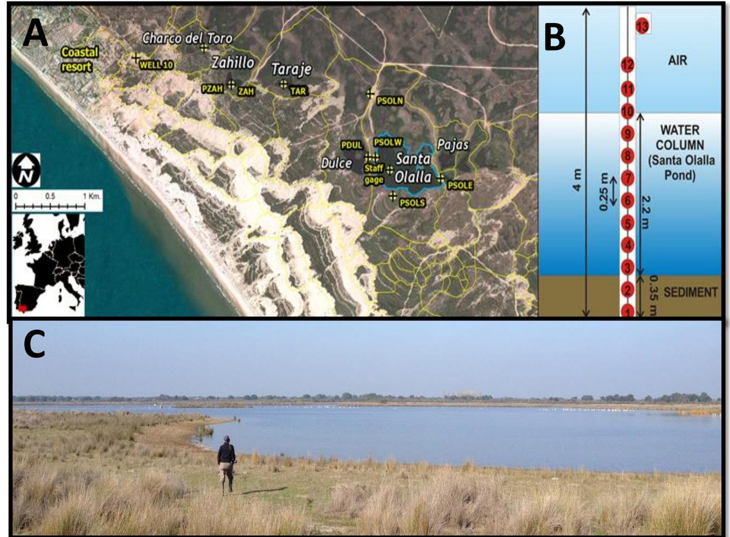
A) Study zone B) Schematic installation of the temperature sensors in Santa Olalla pond B) Santa Olalla pond from the East side (December 2016)
