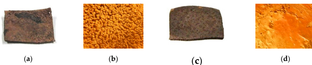
Figure 3. Photograph of electrolytically polymerized MCF rubber: (a) and (b) for cathode side of electrolytically polymerized MCF rubber, (c) and (d) for anode side; (b) and (d) show detail surfaces of (a) and (c), respectively.
