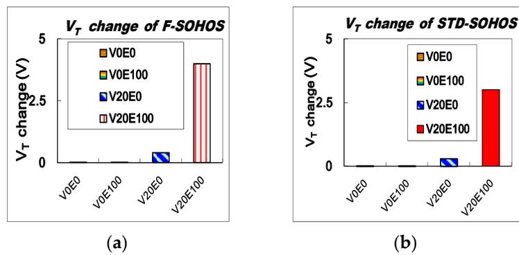
**Figure 4.** (a) The  $V_T$  change of F-SOHOS capacitor devices after various UV irradiation; (b) The  $V_T$  change of STD-SOHOS capacitor devices after various UV irradiation.
