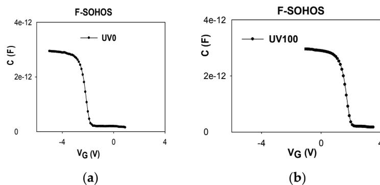
**Figure 2.** This  $C_G$ - $V_G$  curve for an F-SOHOS capacitor device (a) before UV irradiation; (b) after UV TD 100 mW·sec/cm<sup>2</sup> irradiation.
