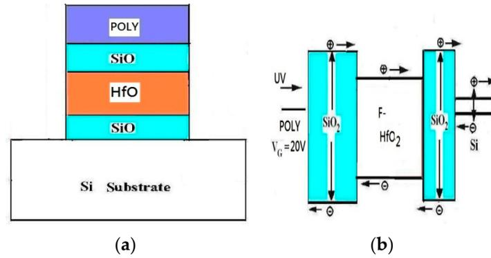
**Figure 1.** (a) Cross-sectional view of an SOHOS capacitor device; (b) Charge generation and trapping in the F-SOHOS capacitor after UV irradiation.
