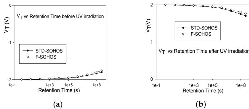
**Figure 6.** The comparison of  $V_T$  vs. retention time for F-SOHOS and STD-SOHOS devices: (a) before UV irradiation; (b) after UV TD 100 mW·sec/cm<sup>2</sup> irradiation under gate PVS 20 V.
