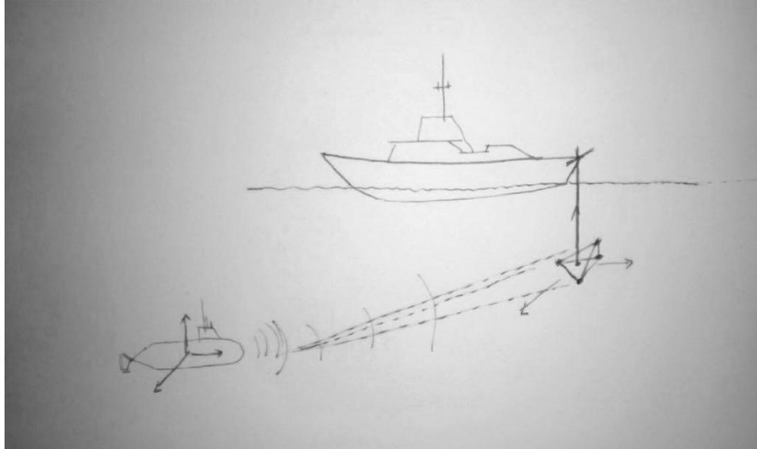
Communications in underwater environments have become a field of research of great interest in recent years. Therefore, the development of submarine sensors have experienced a significant increase in transmission technologies in underwater communication systems. The transmission of information in underwater media can be based on acoustic systems.
