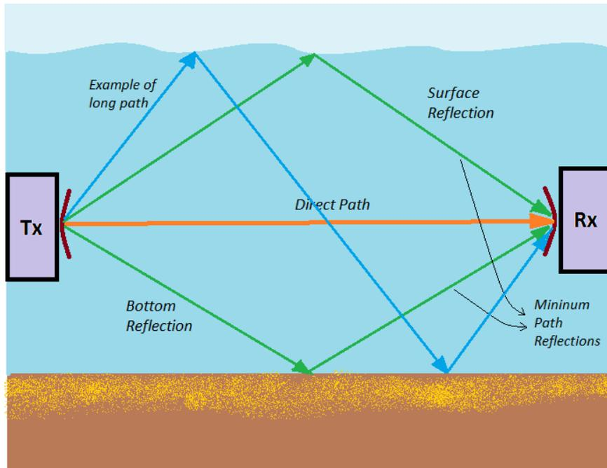
The propagation of the waves in the underwater acoustic channel has important limitations:
