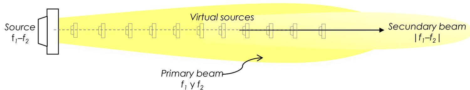
$$p(x, t) = \left(1 + \frac{B}{2A}\right) \frac{p^2 S}{16\pi\rho c^4 \alpha x} \frac{\delta^2}{\delta t^2} \left[ f \left( t - \frac{x}{c} \right) \right]^2 \sim \frac{\delta^2}{\delta t^2} f^2$$
