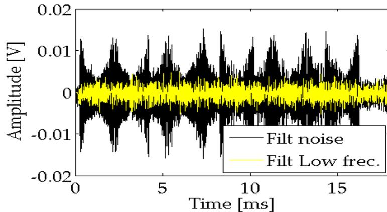
the received signal is filtered at **low frequencies**, → low pass filter of 2 to 60 kHz being applied so as to be able to correlate such signal with the second derivative of the envelope to the square of the signal sent to obtain the secondary beam.
