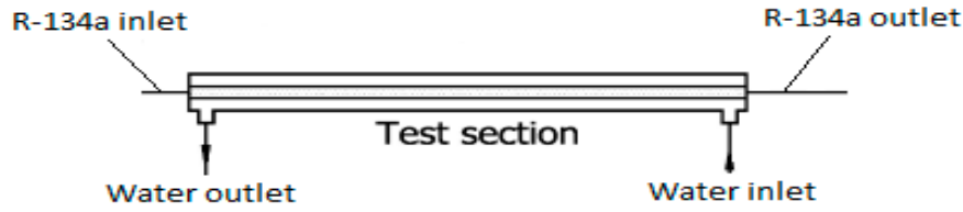
Figure 1. The schematic figure of the micro-fin tube-in-tube heat exchangers [Wongsa-ngam et al., 2002].
