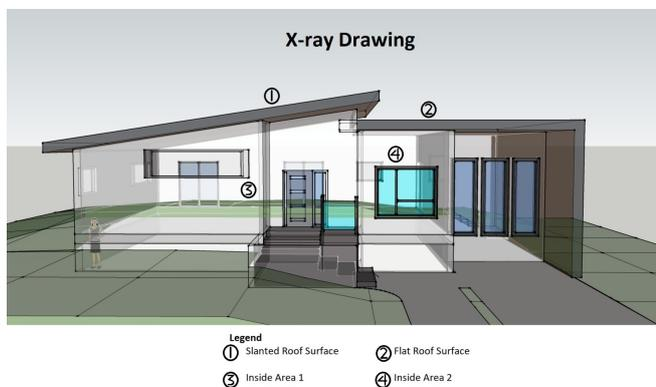
**Fig. 1:** Model house designed with AutoCAD. The geometry facilitate circulation and cooling
