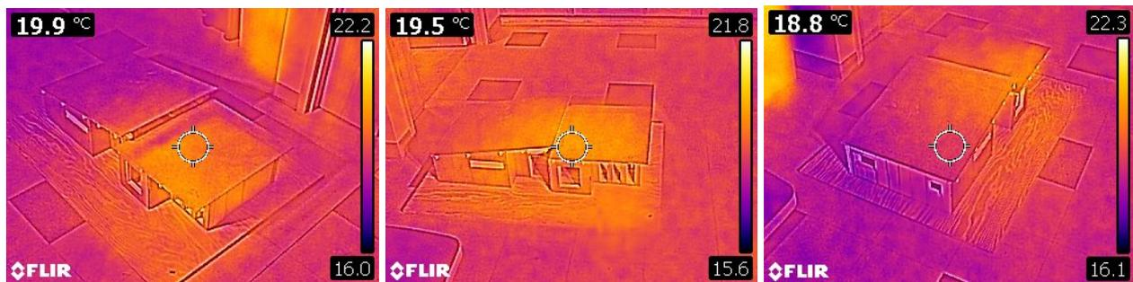
**Fig. 3:** Thermal distribution obtained from the Thermal Infrared Camera for different positions of the source of heat (spotlight emitting about 500W of power). Left-most panel corresponds to the source located to the east, the central panel corresponds to the source located at a center, while the right-most panel corresponds to the source located westward.
