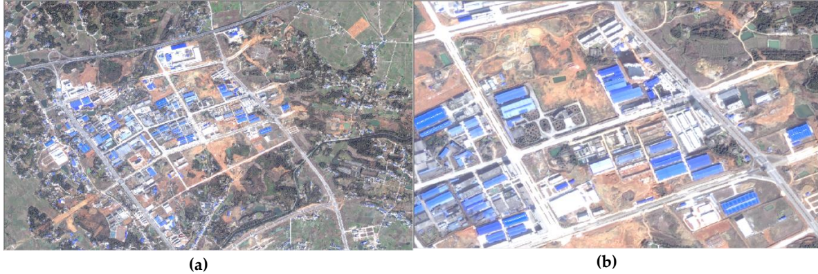
86 Figure 1. The optical distortion on road network of GF-2 image: (a) An area with abnormally whittened 87 road network in center location; (b) magnified detail of (a) .
