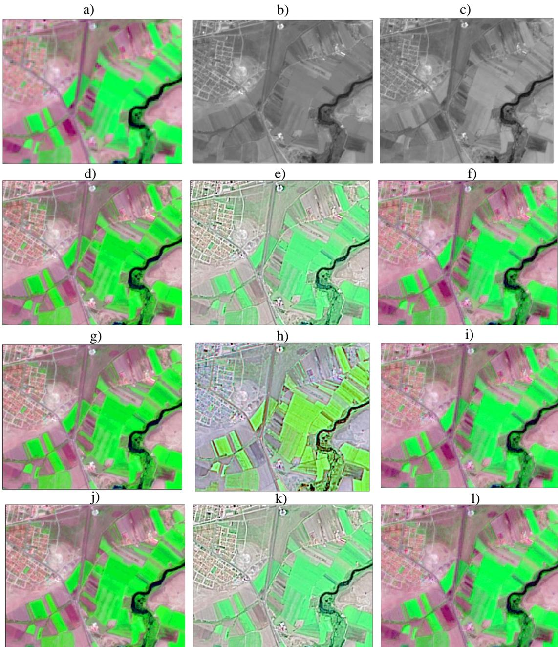
**Figure 1.** Results for a sub-area from the 10.08.2017 image (RGB – 12, 8a, 5); a) 20 m image; b) Pan 1; c) Average value from Band 4 and Band 8; d) IHS – Pan1; e) HPF – Pan1; f) WPC – Pan1; g) IHS – Pan2; h) HPF – Pan2; i) WPC – Pan2; j) IHS – Pan1; k) HPF – Pan1; l) WPC – Pan1.
