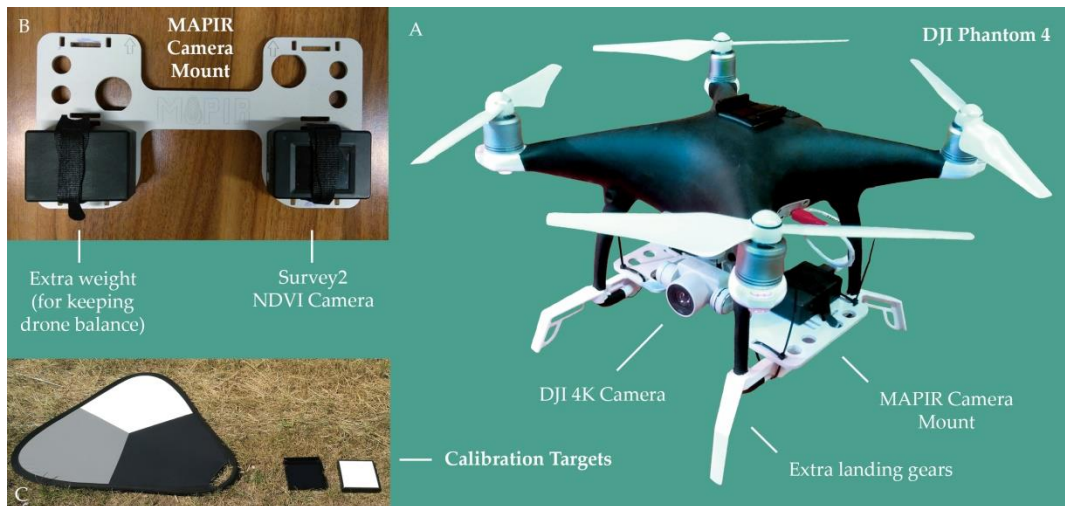
91 Figure 2. UAV platform: (a) modified quadcopter DJI Phantom 4; (b) Camera mount with Survey2 92 NDVI Camera; (c) Calibration targets.
