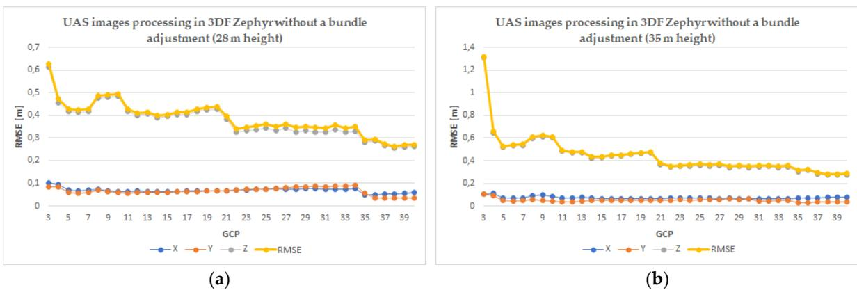
265 **Figure A3.** Errors obtained by performing a Helmert transformation in 3DF Zephyr Pro software when
