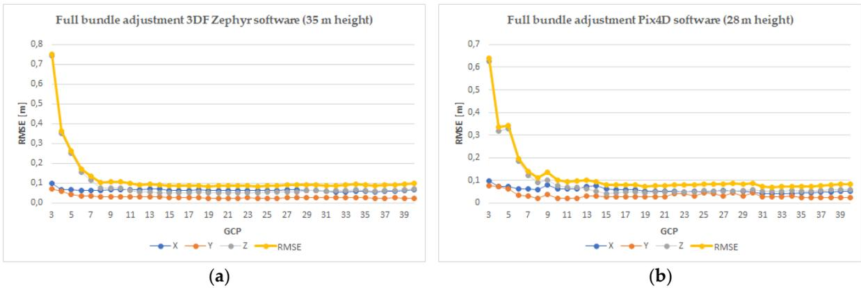
262 **Figure A2.** Errors obtained for 35 m height when using 3 to 40 GCPs along x, y and z directions, as
