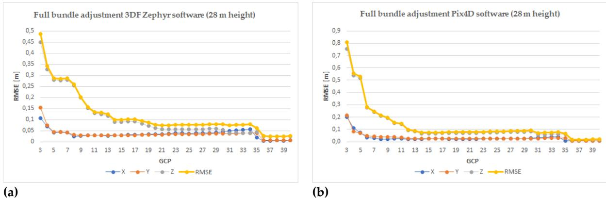
259 **Figure A1.** Errors obtained for 28 m height when using 3 to 40 GCPs along x, y and z directions, as
