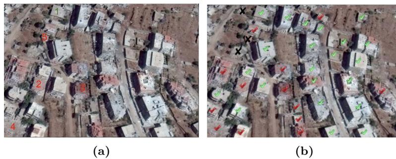
**Figure 2.** Figure 2a shows 5 labeled buildings investigated in details in Table 1 and Figure 2b shows building damage assessment results of the proposed algorithm.
