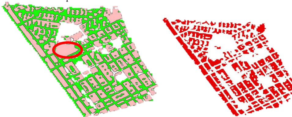
Figure 6. Final detection results (Left: Buildings from SAR (pink), Göktürk(green), Right: Intersection result)
