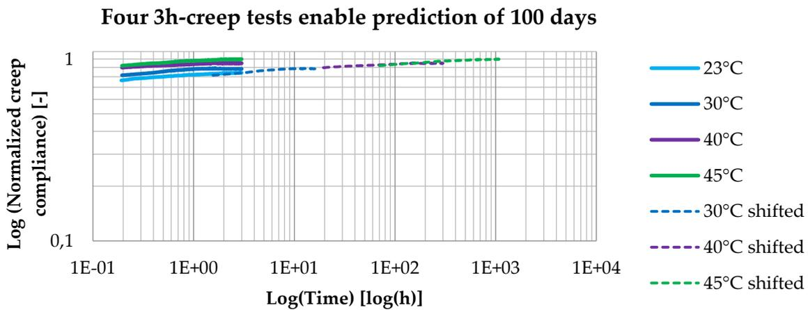
**Figure 6:** Master curve for PA6 created from tensile curves according to a load of 1 % of the tensile strain at a strain rate of  $10^{-5}s^{-1}$
