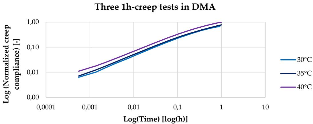
**Figure 5:** Creep curve of PA6, performed from 23 °C until 45 °C in 5 °C steps created from DMA test with a load according to 0.1 % of the tensile strain at a strain rate of  $10^{-5}s^{-1}$
