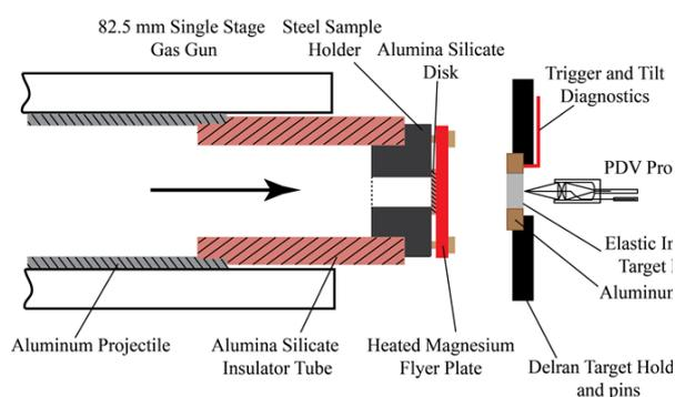
**Figure 1 (b).** Schematic of the elevated temperature normal plate impact experimental configuration used in the present study
