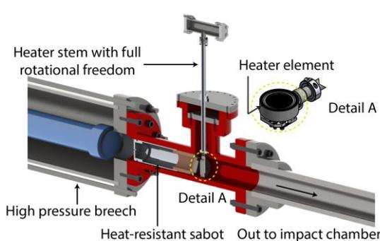
**Figure 1 (a).** Schematic of the custom designed heater system with axial and rotational degrees of freedom at the breech-end of the gas gun
