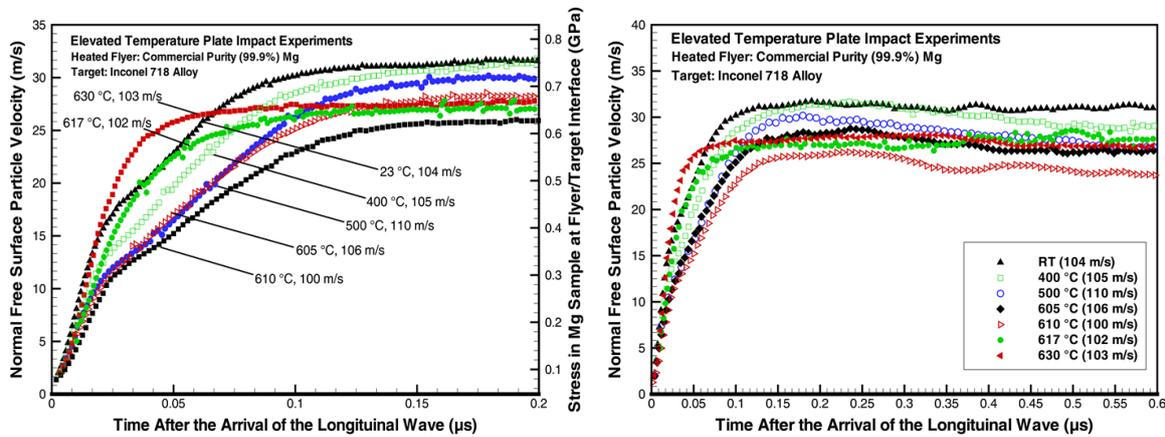
**Figure 2 (a).** The onset of incipient plasticity in commercial purity 99.9% polycrystalline magnesium samples in the temperature range 23 to 630 °C.
