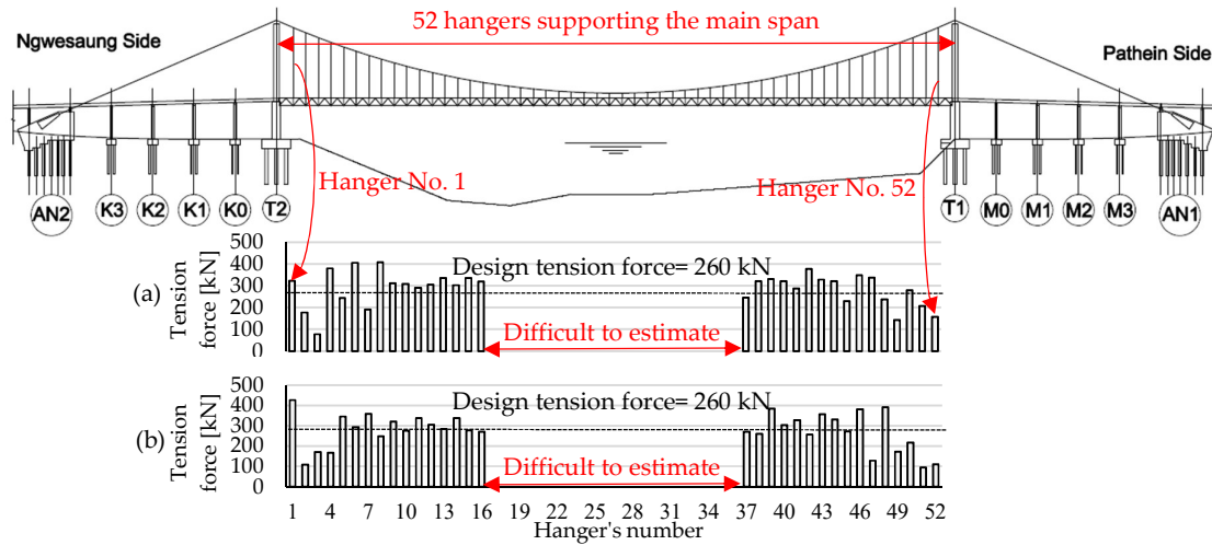
Figure 8. Hangers' tension force distribution of Pathein Bridge. (a) Tension force of hangers of upstream; (b) Tension force of hangers of downstream.
