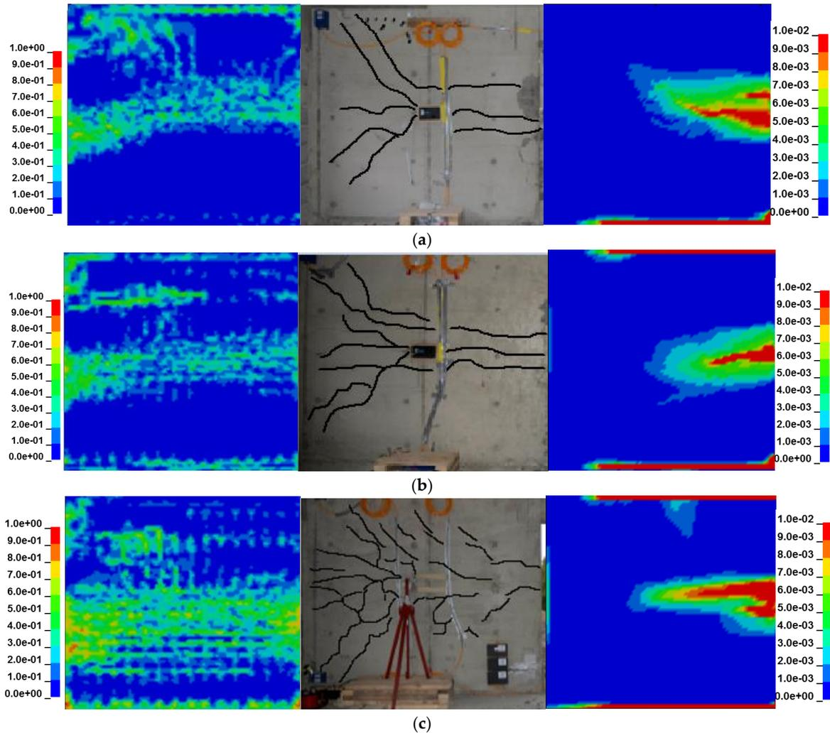
**Figure 6.** Local damage on the rear side of the front wall from the solid element model, the experiment and the structural model, for Level 3 (a), Level 2 (b) and Level 1 (c). In the solid element model red elements indicate failed elements due to either ductile or brittle damage. In the structural element model red areas indicate where reinforcement bars have higher plastic strains than 1%.
