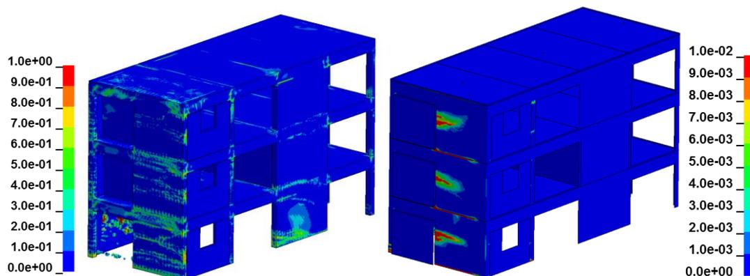
**Figure 4.** Global damage on the solid and the structural element model. In the solid element model red elements indicate failed elements due to either ductile or brittle damage. In the structural element model red areas indicate locations where reinforcement bars have higher plastic strains than 1%.
