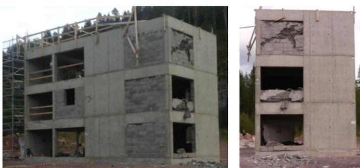
Figure 2. Global damage of the three-story building after the air-blast from front side view and front view.
