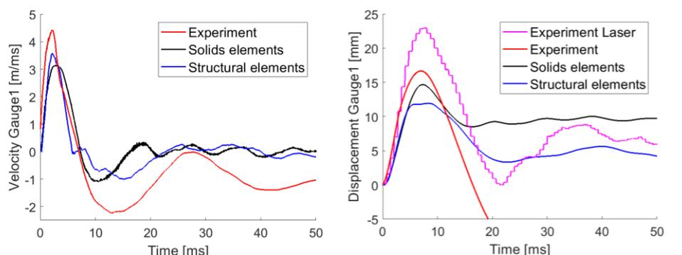
**Figure 5.** Velocity and displacement in horizontal direction at gauge A1 from the experiment and the numerical simulations with solid and structural elements for the first 50 ms.
