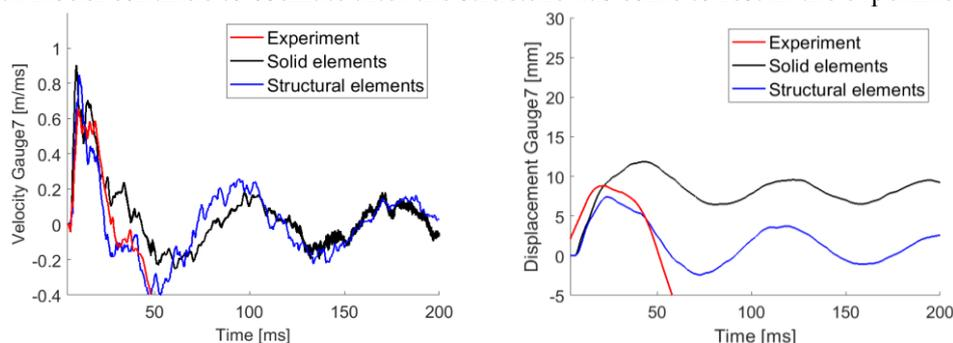
Figure 3. Velocity and displacement in horizontal direction at gauge A7 from the experiment and the numerical simulations with solid and structural elements.
