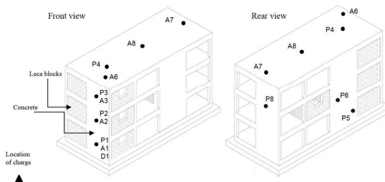
**Figure 1.** Isometric view of building. Location of pressure gauges, accelerometers, the displacement gauge and the explosive charge [6].
