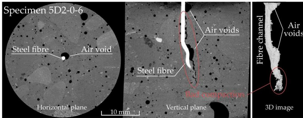
**Figure 2.** Micro-CT scans of specimen 5D2-0-6: horizontal and vertical plane through the specimen’s centre and a 3D outer surface image of the fibre channel and connected air void after fibre pull-out.
