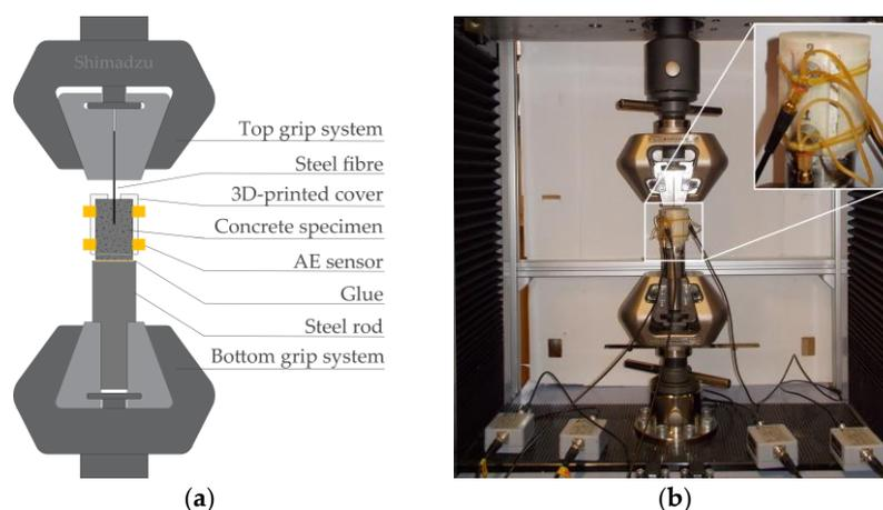
**Figure 1.** Experimental setup: (a) Schematic overview; (b) Photograph with detail of concrete specimen with 3D-printed cover and AE sensors.
